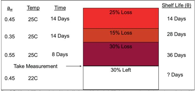
Figure 6. Real-time shelf life of a product as determined by the cumulative loss in shelf life due to exposure to varying temperatures and water activity levels. Total shelf life is determined by summing the number of days spent at the various conditions plus the remaining days of shelf life as predicted based on the expected storage conditions and the percentage of shelf life remaining.
