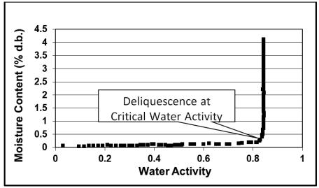
Figure 2. Moisture sorption isotherm showing the deliquescence of a crystalline material.
