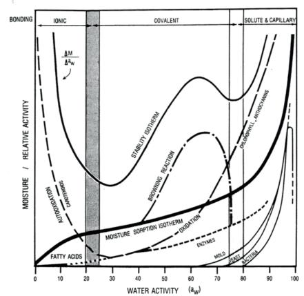
Figure 5. Water activity stability diagram showing the impact of water activity on various degradative reactions that shorten shelf life.
