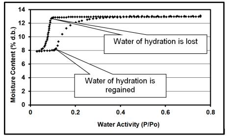
Figure 1. Gain and loss of waters of hydration in a crystalline material.
