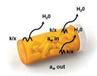
Figure 8. Diagram showing the movement of water in or out of a packaging material as determined by the difference in water activity inside and outside the packaging and the water vapor permeance (k/x) of the packaging material.
