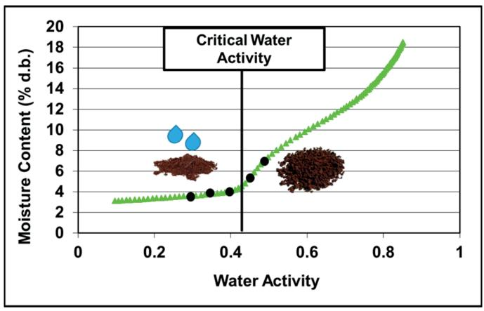
Figure 3. Moisture sorption isotherm indicating the critical water activity for a glass transition. Below the critical water activity, the product remains stable. Above the critical water activity, the product becomes unstable and shelf life is reduced.
